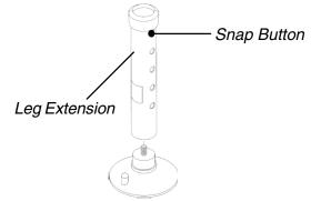
FIGURE 2 - REMOVING THE EXISTIING LEG EXTENSIONS
